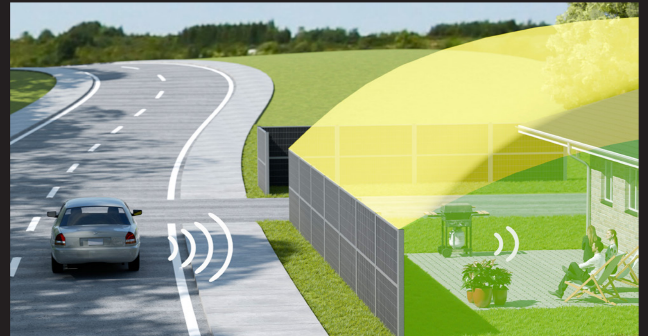
An absorbing fence reduces noise by soaking up sound waves, creating a quiet environment.
