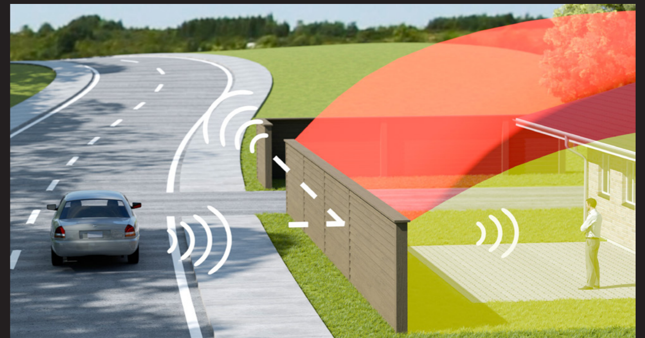
A reflecting fence bounces sound waves back toward the source, limiting noise reduction on the far side.
